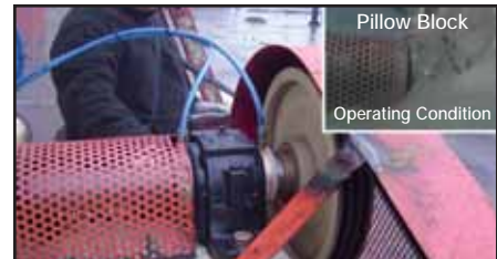
LabTecta-OAP-PB™ installed on a Pillow Block duty
