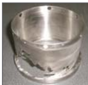
Abrasive single cartridge sleeve damage from inboard seal leakage
