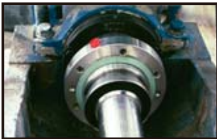
CVSD™ installed on a Slurry pump.
