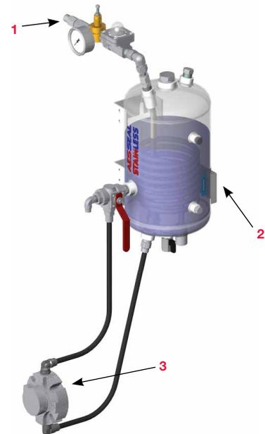
1. Water from the plant water line enters the system.
