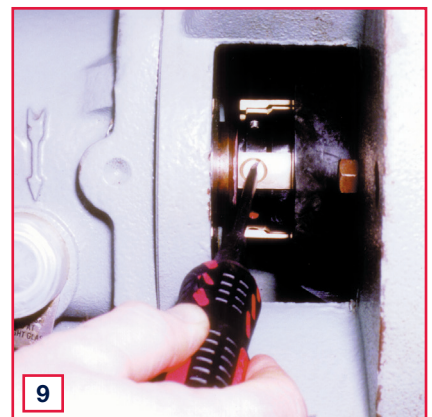
9 Unscrew and remove the setting clips. Spin the shaft by hand, listening for shaft binding. Pipe up to inlet & outlet ports on the pump chamber. Ensure the barrier fluid is present and the seal is primed before start up.
