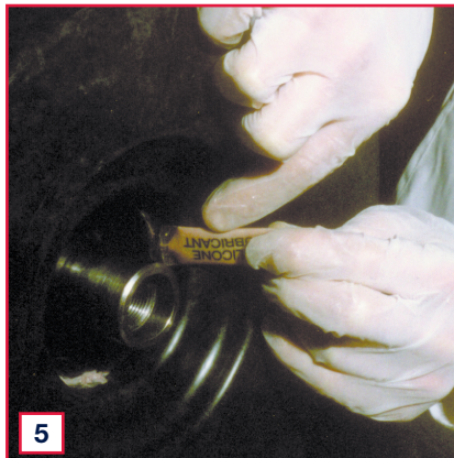
5 Apply grease to the recess on the pump where the inboard stationary is seated.
