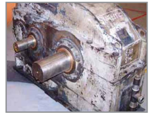
LabTecta® installed on a Falk gearbox
