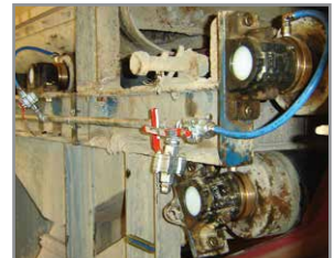
LabTecta-OAP-PB™ installed on mining conveyor belt
