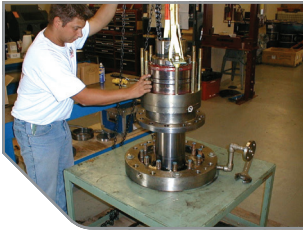
$50,000 mixer bearing destroyed by rainwater penetrating a $20 lip seal (Case Ref: 3459)
