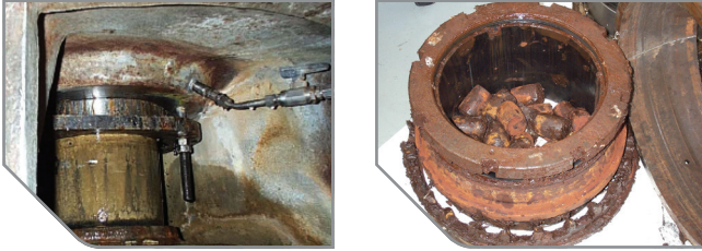
Water contamination on a continuous digester prior to a LabTecta®66 being installed (Case Ref: 3232)
