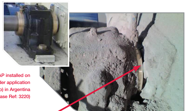
LabTecta®66OAP after three months running. Note: Air purge keeps the dust away from the stator to rotor interface
