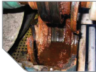
Pillow block without LabTecta®66PB technology (Case Ref: 3217)
