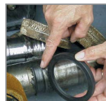
Shaft damage from a lip-seal
