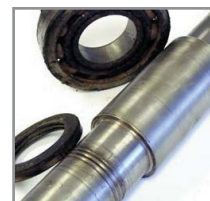
Shaft damage from a labyrinth seal
