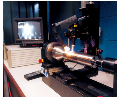
CNC outside diameter bellows welding operation
