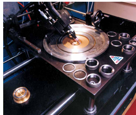
CNC inside diameter bellows welding operation.
