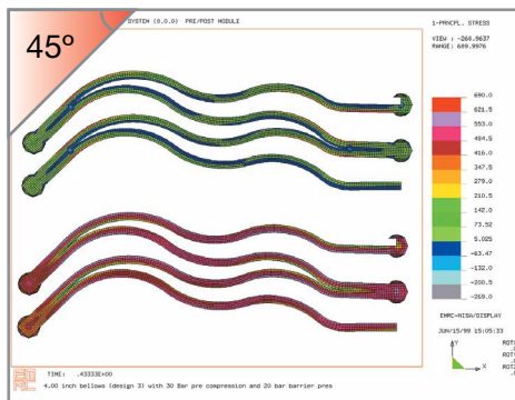
Optimized bellows convolution design.
