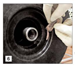
f). Apply the grease (supplied) to the recess on the pump where the inboard stationary 'O' ring (6) is seated (see figure 6).
