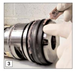
**c).** Apply the grease (supplied) to the inboard rotary 'O 'ring, (see figure 3), again ensuring that the grease covers the full circumference of the seal.
